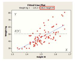
The blue line is Y = -114.3 + 106.5X. (*X* in meters, *Y* in kg.) Best linear fit: Linear Regression.
